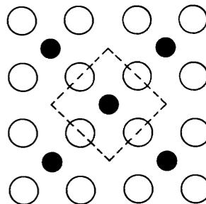
FIGURE. Suggested structure of silver ketenide (I) projected on to *ab* plane. Light circles denote silver atoms in plane of page (Ag–Ag = 2.84 Å, interplanar spacing 5.846 Å), and dark circles denote C-1 (of linear C<sub>2</sub>O groups) lying below this plane and eclipsing C-2 and O.
