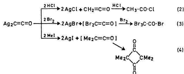
Treatment of ketenide (I) with an excess of Br<sub>2</sub> in CCl<sub>4</sub> at 20° (Equation 3) gives tribromoacetyl bromide (>90%). Tetramethylcyclobutane-1,3-dione is produced by the reaction with MeI in octane at 90°. These reactions are consistent with the formulation of (I) as a disilver(i) ketenide in which both silver atoms are covalently linked to the terminal carbon of the ketenide group.
